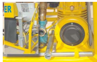
1. Cleaning tools mounted on machine
