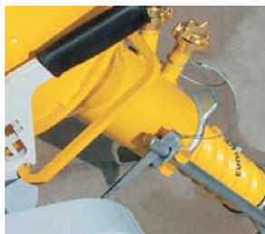
Stator fixing system.
